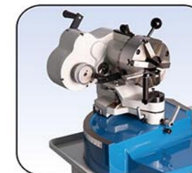
Patent No. 135236 Double cams. It can grind tool of 1/2/3/4/6 Flutes.
